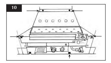
6.14 Turn the appliance off, disconnect the "U" gauge and replace the sealing screw. Relight the appliance and check the sealing screw for leaks.
